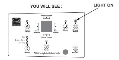
**Note:** This feature is a reminder to clean the Air Filter (See Care and Cleaning) for more efficient operation and cooling. The LED (light) will illuminate after 250 hours of operation. To reset after cleaning the filter, press the "Check Filter" button and the light will go off.
